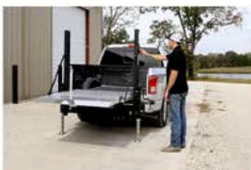
4 Load truck and raise the platform
